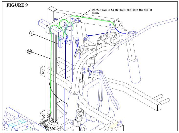
Install the **NEW** 110-3/4" CABLE ASSY (16) using the following steps:
